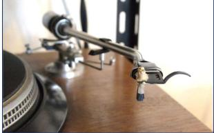
Attach the carbon fiber brush to the tonearm just like a cartridge.
