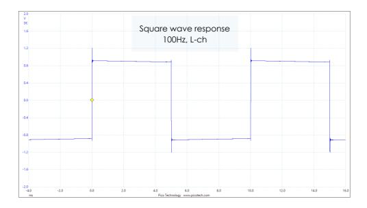
The waveform is slightly slanting. That implies the response in very low frequency is low. MR-2000S probably has an output capacitor (AC coupling).
