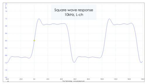
There seem to be overshoot and undershoot, but these peaks are caused by lack of very high frequencies. The ringing is so small. This well-shaped waveform explains high sound quality of MR-2000S.
