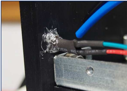
The LED fixed with hot melt adhesive
