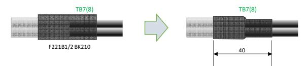
(4) Slide the shells of the RCA plugs (P11-12) onto the wires
