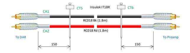
(2) Tie cable assys CA1-2 with cable tie CT8-10 (Insulok AB100-W-100) at intervals of 300mm.
