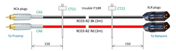
(2) Tie cable assys CA5-6 with cable tie CT23-30 at intervals of 300mm.
