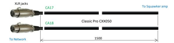
(2) Cut sleeving (FRN0.25TW) into 1.2m (SV4) and slide it onto the cabel assys CA17-18
