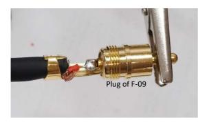
(7) Solder the white wire and shield to the cold terminal, and crimp the sheath of the cable
