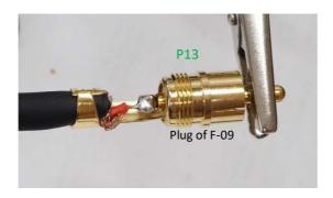
(5) Solder the white wire and shield to the cold terminal, and crimp the sheath of the cable
