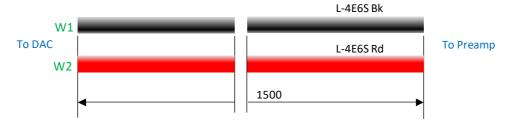
(2) Cut sleeving (FRN0.25TW) into 1.2m and slide it onto the wires W1-2
