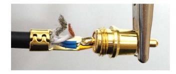
(7) Solder the white wires to the cold terminal
