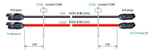
(2) Tie cable assys CA9-10 with cable tie CT36 at intervals of 350mm.
