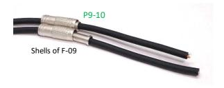
(5) Strip the insulators of the wires
