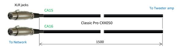
(2) Cut sleeving (FRN0.25TW) into 1.2m (SV3) and slide it onto the cabel assys CA15-16
