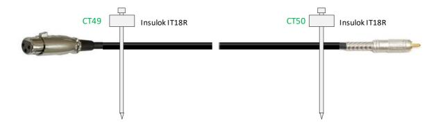
(8) Make pin-3 (cold) of the XLR connectors open Dismantle the XLR connectors. Cut the white wire off the pin-3 (cold). Refix the connector.
