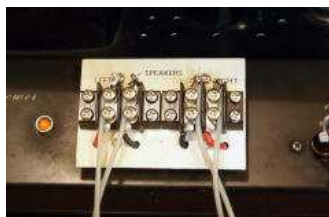
Connection of the speaker cable (the woofer amp side)
