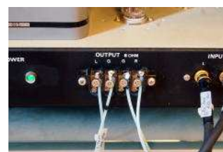
Connection of the speaker cable (the tweeter amp side)
