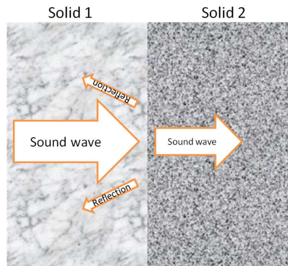
Sound propagation from a solid body to a solid body Reflection is small, most sound goes into the other body.
