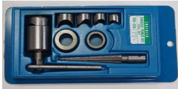
Chassis punch set for round cutouts (Engineer TR-05)
