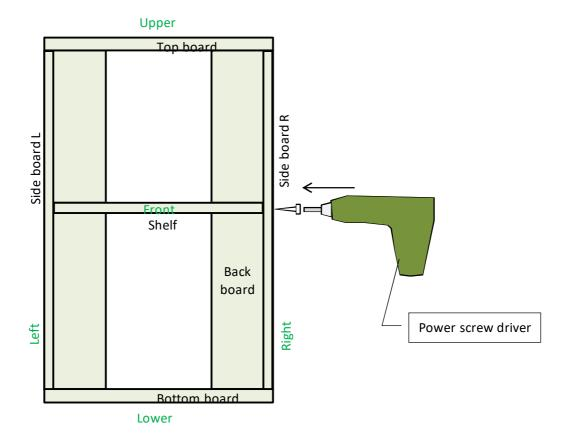
(13) Place bottom board (BD19), side boards (BD20-21), front board (BD22) and back board (BD23) on work bench
